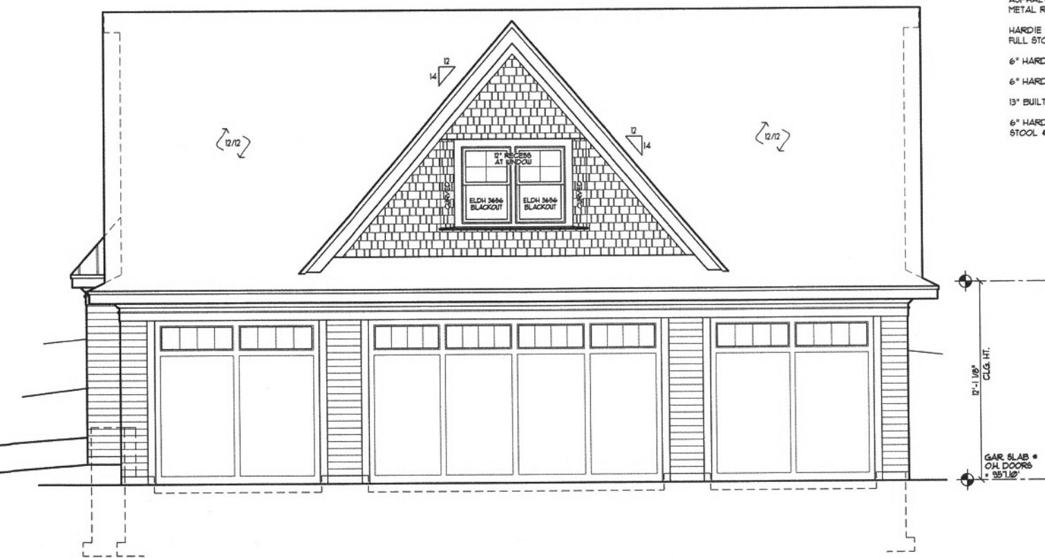
1 DETACHED GARAGE FRONT ELEV. SCALE: 1/4"=1'-0"
